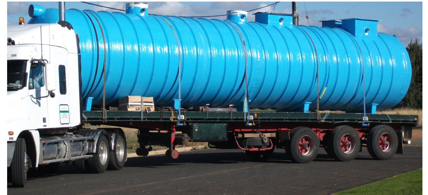
Horizontal Fibreglass Pump Station
